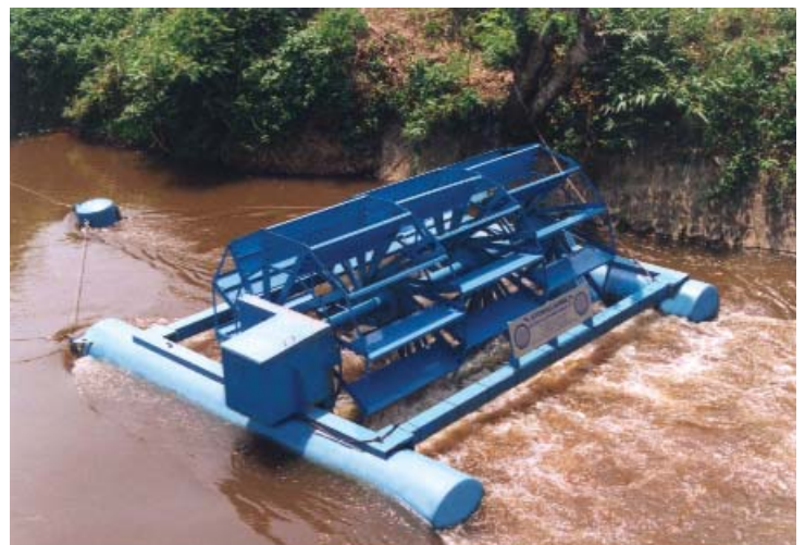
Hydrolienne of Kikimi (30 km from Kinshasa) on the river Ndjili Photo © Rutten SA
